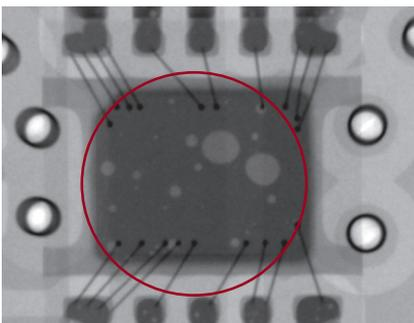
Void in a surface solder joint
